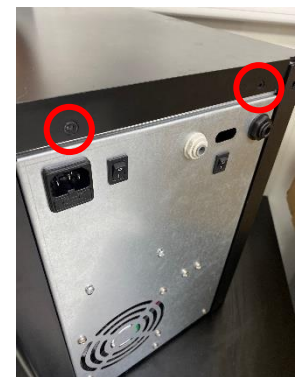
9. Screw back on the two screws onto the back of the lid component.
